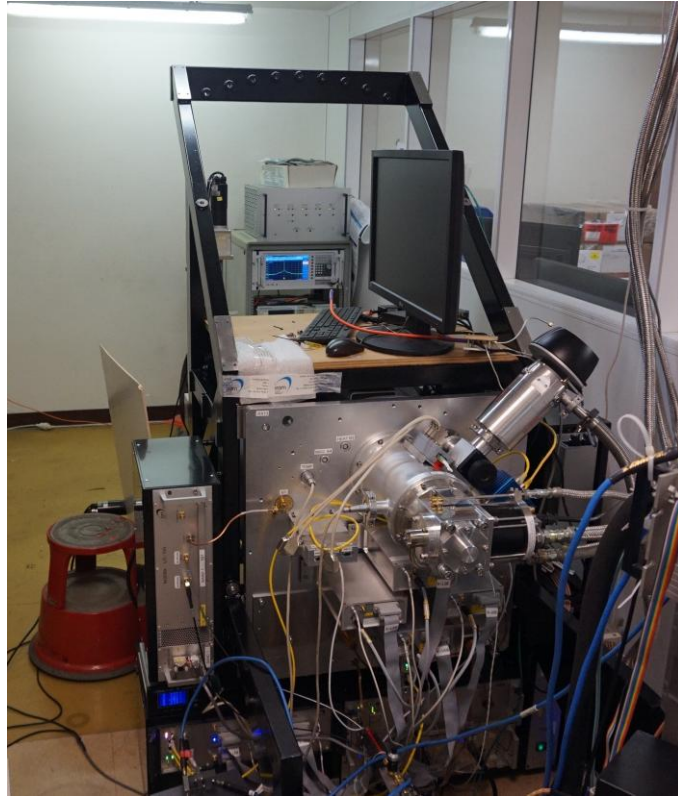
Figure 5: In the Grenoble laboratories, the full receiver is installed in the same support frame which will then be connected to the telescope receiver cabin interface ring. Full characterizations are performed in this configuration. Detail of the receiver design can be found in [4]
