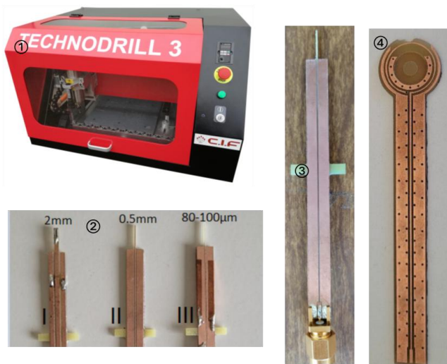
Figure 2: CNC milling used, spatial resolution, electric and magnetic probes
